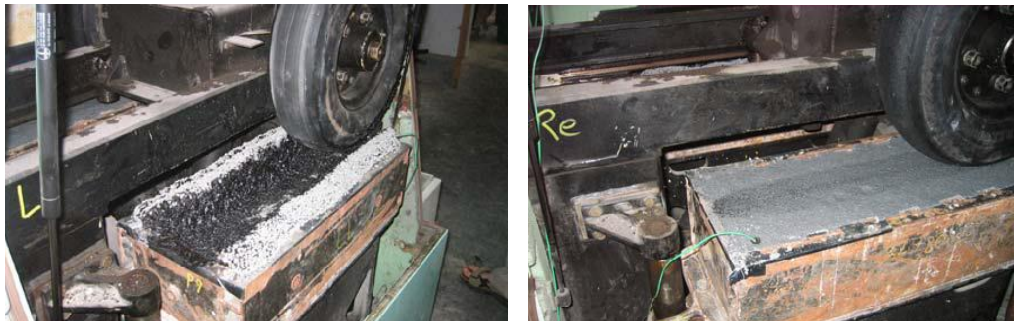
Figure 13: Comparison of flexible plug materials after rutting test per EN 12697-22 at 60°C. (Left: Common asphalt plug after 100 cycles. Right: PU material of described joint after 30,000 cycles)
