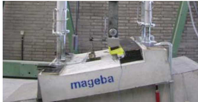
Figure 6: Testing of the joint shown in Figure 3 (incl. noise-reducing surface plates as shown in Figure 5)
